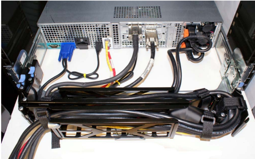
Figure 5: Left-Side Mounted CMA Installation
